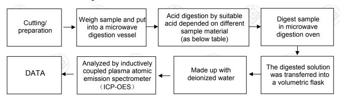
2. Test Flowchart for Cr(VI) content (For non-metal material)
