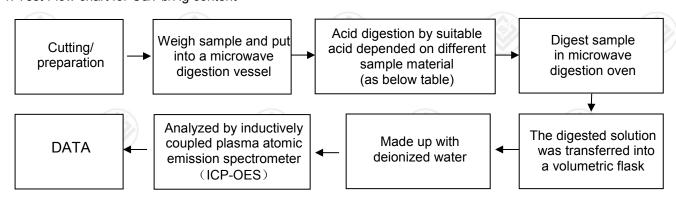
2. Test Flowchart for Cr(VI) content (For non-metal material)
